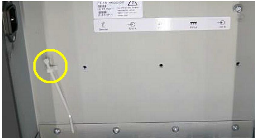
5. Insert the DVI cable directly into the DVI socket. Only Dual Link DVI cables of a correspondingly high quality may be used.
