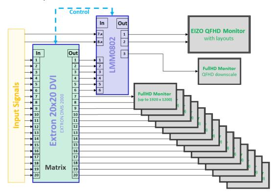
Fig.: LMM0802 with Extron 20x20 DVI matrix (example with 6 signals from the matrix to the LMM)
