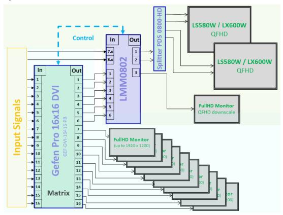
Fig.: LMM0802 with splitter and Gefen 16x16 DVI matrix (example with 6 signals from the matrix to LMM)
