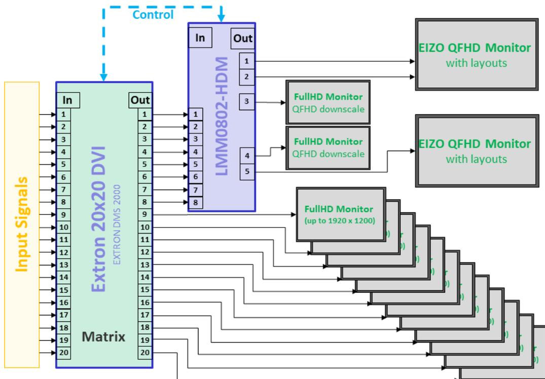
Fig.: LMM0802-HDM with Extron 20x20 DVI matrix (example: eight matrix outputs connected to the LMM)
