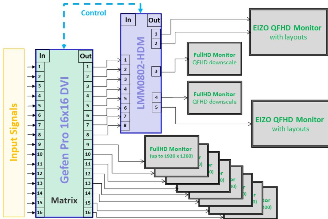
Fig.: LMM0802-HDM with Gefen matrix (example: eight matrix outputs connected to the LMM)
