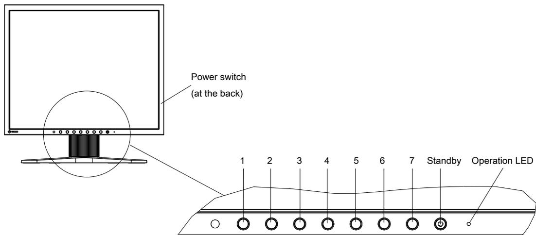
The OSD keys and the operation LED are located on the front of the monitor.
