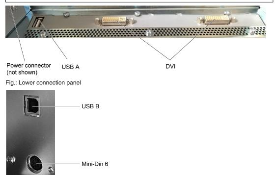
Fig.: Side connection panel
