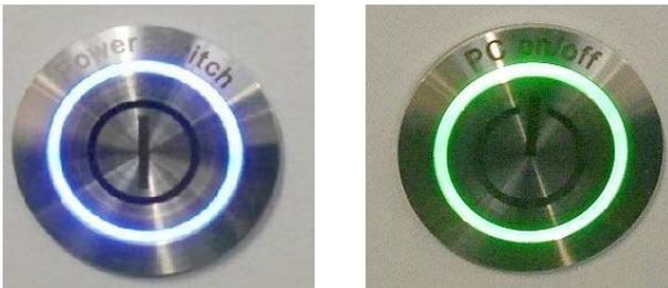
3. Press the green-bordered switch labeled “PC on/off”.
