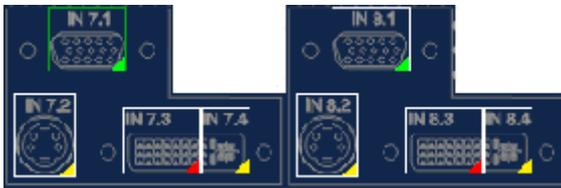
If you double-click with the left mouse button the analog video input IN7.1, IN7.2, IN7.4, IN8.1, IN8.2, or IN8.4 that is to be configured, the "Video input configuration" dialog window is displayed.
