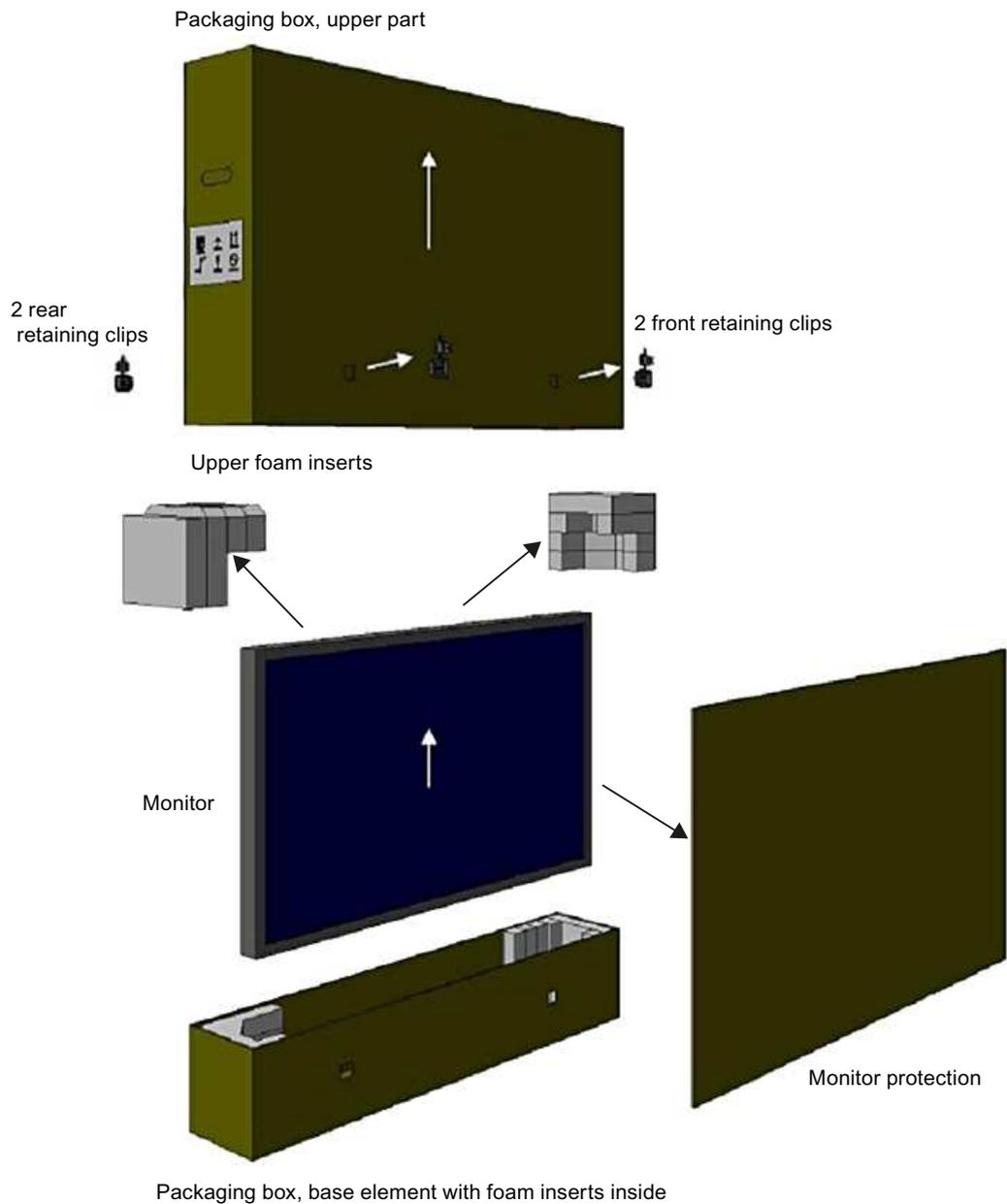
Fig. 1: Monitor packing (schematic representation)
